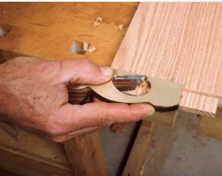
PHOTO C: A shoulder plane makes neat work of trimming tenon shoulders.
