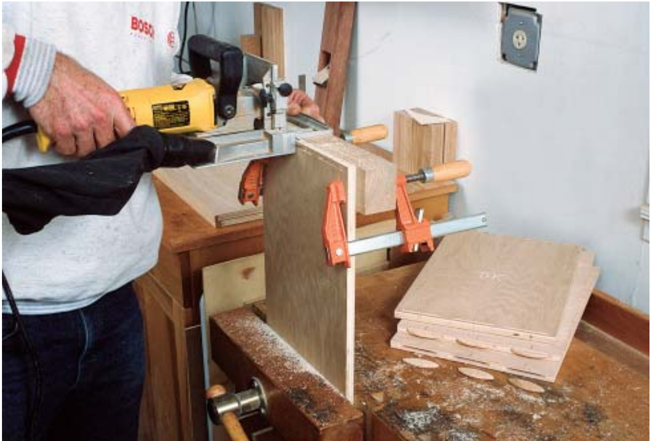
PHOTO G: Square scrap clamped to the case pieces provides bearing for the biscuit joiner fence, preventing angled slots.
